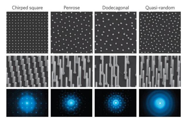
Two-dimensional silicon wire patterns for solar applications, ranging from ordered (left), to quasi-crystalline and hyper-uniform (right). Top row: scanning electron microscopy images from a top-down perspective. Middle row: scanning electron microscopy images viewed at an angle of 20°. Bottom row: transmitted diffraction patterns of polymer-embedded wire arrays on a quartz slide, observed at a wavelength of 488 nm.
